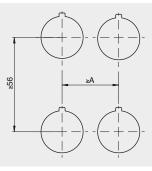
3-slot mounting adapter A=30 mm
