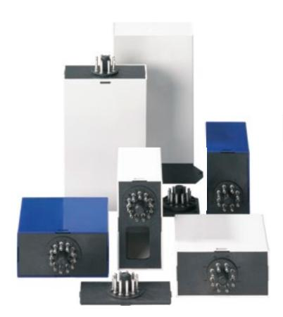
8 or 11 pole Plug-Socket-Enclosures MBRE for varied application options in control technology. Two different installation depths and guide grooves in the cover provide scope for freedom of design. The top part of the enclosure is made of ABS and the base is Noryl.
