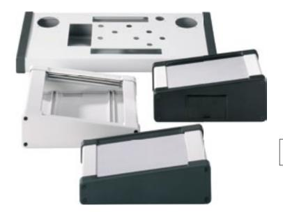
TAST-Enclosures made of extruded aluminium profile serve as desk, wall or machine enclosures. They are preferably used as keyboard, operating elements or displays. The dimensions and groove guides in the base allow convenient assembly of PCBs in European card format or other electronic components. The aluminium front plates are 2 mm thick and silver anodised. The end caps are made of impact-proof ABS.
