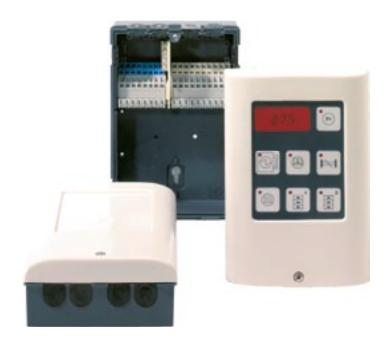
The MBRS-19 Control-Enclosure is a completely new enclosure concept and allows simple connection technology for up to 19 special cage clamp terminals from the company Wago. These can be clipped directly onto the enclosure base. A corresponding terminal strip contacts the board, which can easily be mounted into the enclosure cover.
