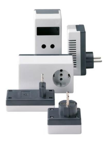
Electronic-Connector-Enclosures with different plug versions made of flame-resistant and impact resistant Polystyrene are frequently used for industrial power packs and chargers. Plugs in Schuko, European, Swiss and French versions are available as options. Excellent stability is achieved with the groove and spring sealing and the base parts that open to the side allow fast and uncomplicated assembly of construction elements.
