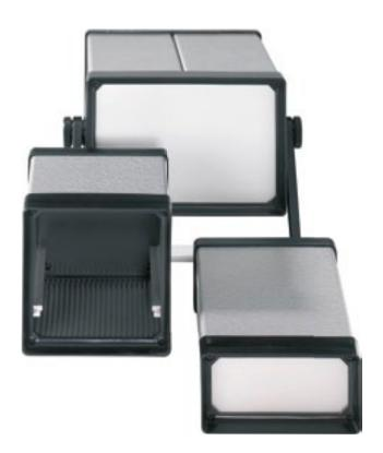
KDCA-Enclosures are made of two aluminium u-profiles and are primarily used as command, desk or wall enclosures. With the practical Europe card insert, varied application options result. The aluminium front plates are 1 mm thick and silver anodised. The back wall and front frame are made of impact-proof ABS.
