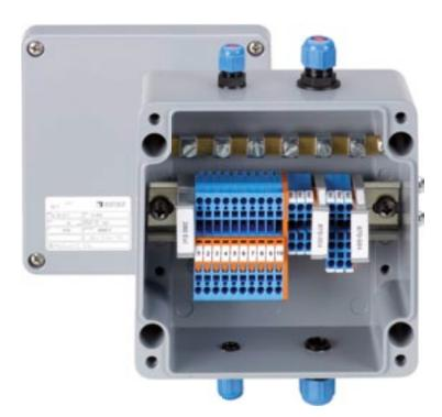
MULTI-BOX Aluminium-Ex i junction boxes are conform to all requirements for installation fields where explosive concentrations of gases, steams and dusts can appear (zones 1 and as well as 21 and 22). MBA-Ex i enclosures can be used in the temperature classes T4 up to T6.
