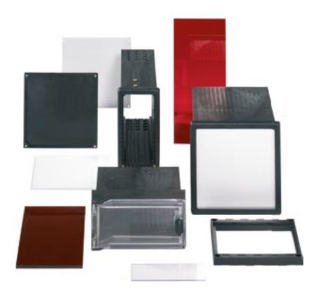
Instrument-Panel-Enclosures MBS are made of fibre glass reinforced Noryl and have been specially developed for measurement and display technology in accordance with DIN 43700. The circumferential guide grooves inside the enclosure result in universal applications for circuit board installations. A front frame for the use of different front plates, such as aluminium or fibre glass, is also available.
