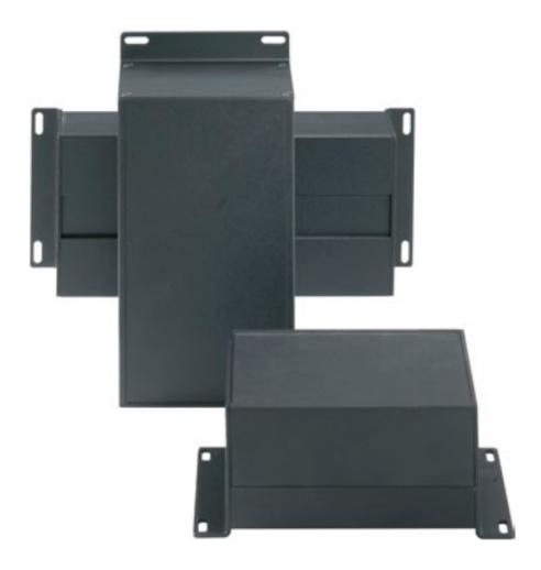
ETP-Enclosures are made of two assembled aluminium u-profiles and are primarily used as wall or control enclosures. Connection of the profiles with a groove/spring system and aluminium end caps give this enclosure high stability. The inner guide grooves allow simple assembly of PCBs and other components. Direct assembling on mounting rails (TS 35) is possible with an adapter.
