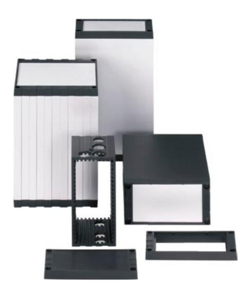
MBAL-Enclosures made of extruded aluminium profile are preferably used for small controls. The inner circumferential guide grooves allow simple assembly of PCBs and other components. The enclosure can be used in line with EMC without further treatment. Front frames and end caps are made of fibre glass reinforced Polyamide.
