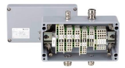
MULTI-BOX Aluminium-Ex e junction boxes are conform to all requirements for installation fields where explosive concentrations of gases, steams and dusts can appear (zones 1 and 2 as well as 21 and 22). MBA-Ex e enclosures can be used in the temperature classes T4 up to T6.
