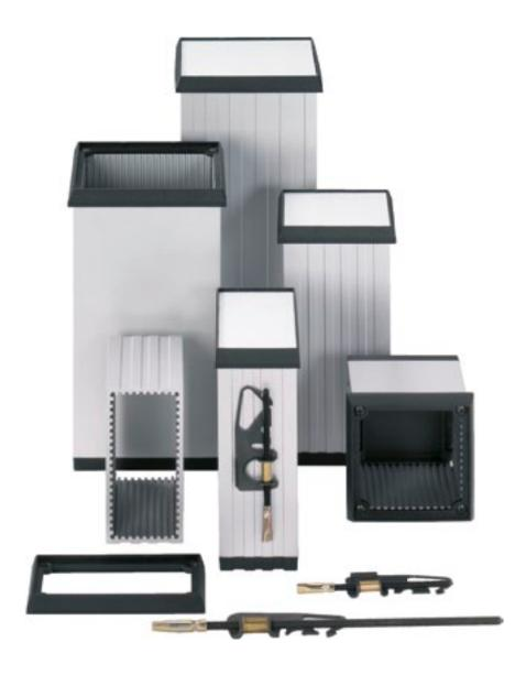
MBAS-Enclosures made of extruded aluminium profile are preferably used for control and display tasks. The inner circumferential guide grooves allow simple assembly of PCBs and other components. The enclosure can be used in line with EMC without further treatment. Front frames and end caps are made of fibre glass reinforced Polyamide.
