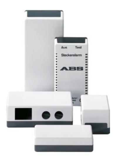
Electronic-Enclosures MBPO in a shapely design made of impact resistant Polystyrene are particularly suited to "packaging" small controls and desk units. Excellent stability is achieved with the groove and spring sealing and the base parts that open to the side allow fast and uncomplicated assembly of construction elements.
