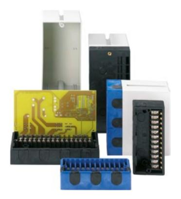
Plug-Card-Enclosures MBZA with goldplated contacts offer the possibility of direct contacting between the circuit boards and connection terminal. The enclosures are used in different areas for small control systems. The enclosure cover is made of Polystyrene, and the base of fibre glass reinforced Polyamide.
