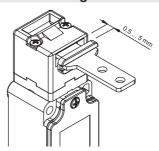
This switch has a wide backlash of the actuator into the head (4,5 mm) for an easier installation. With closed door, check that the actuator doesn't knock straight against the head of the switch; it must be in the adjustment zone (0,5...5 mm)
