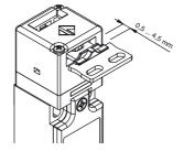
This switch has a wide backlash of the actuator into the head (4 mm) for an easier installation. With closed door, check that the actuator doesn't knock straight against the head of the switch; it must be in the adjustment zone (0,5...4,5 mm)
