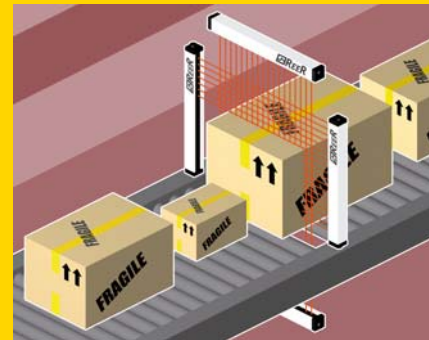
Two-dimensional detection of objects in transit on conveyor systems with use of 2 light curtains
